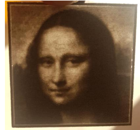
MJF part printed at 45° with a minimum thickness of 0.08mm
